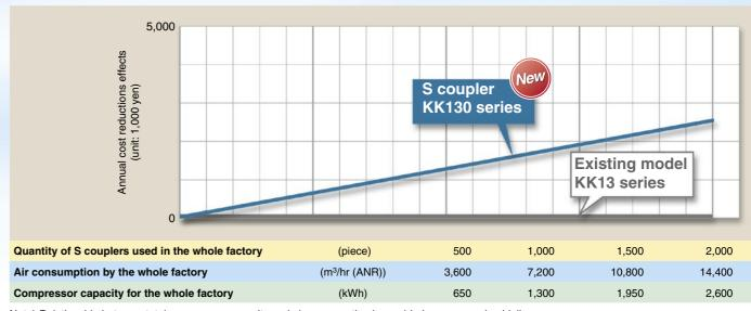
Note) Relationship between total compressor capacity and air consumption is provided as a general guideline.
